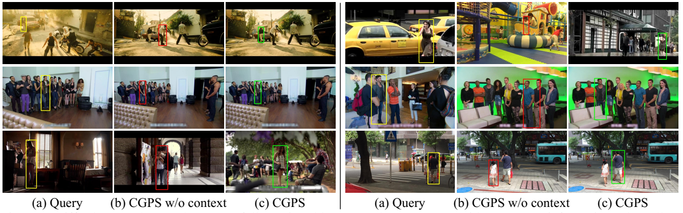
Figure 4: Difficult cases that can be successfully retrieved by CGPS, but not CGPS without context information. The yellow bounding boxes denote the queries, while the green and red ones denote correct and incorrect top-1 matches, respectively.
