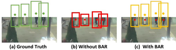
Figure 4: Visualization detection results at the boundary. (a) Ground-truth bounding boxes. (b) The incomplete bounding box prediction. (c) The bounding box prediction with boundary-aware regression (BAR). The red points represent the anchor centers and green/yellow points represent centers of the bounding boxes.
