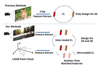
Figure 1: Motivation. SimIPU is designed on both the 2D image plane and the 3D space. Intra-modal module learns the spatial-aware representation with point clouds. Intermodal module transfers the capability of extracting spatial-aware representations to the image-feature extractor. 'CL' is the abbreviation of the contrastive learning.
