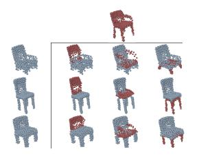
Figure 4: Parts mixing in the chair category with M = 3. Far left: ground truth point clouds, top: reference point cloud. Remaining: from left to right, back, base, and legs for ground truth points are mixed by corresponding parts in the reference one via mixing their disentangled latents.
