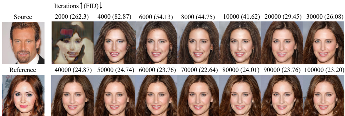
Figure 2: Visualizations and Fréchet Inception Distance (FID) variations of StarGAN v2 on CelebA-HQ dataset with the increase of training iterations. The first column shows the source image and the reference image of a specific image synthesis task, while remaining columns are images generated by intermediate models at different training iterations. The parentheses above each generated image gives FID score at corresponding training iterations.
