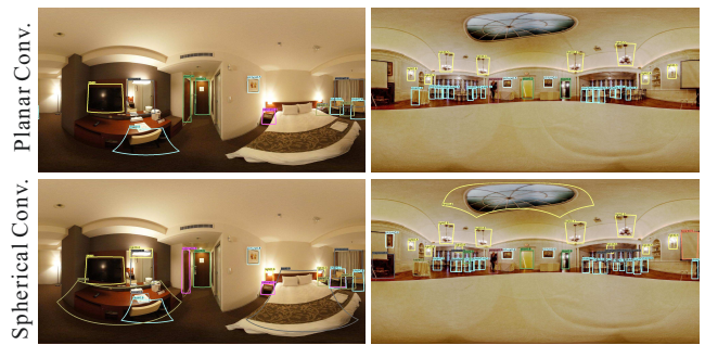
Figure 8: Compared with planar convolution, spherical convolution can detect more seriously distorted objects.
