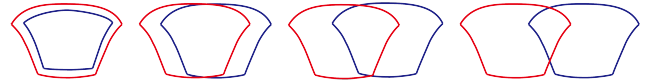
Figure 4: The intersection between two spherical rectangles in unrolled spherical images may have different shapes. From left to right, the intersection is spherical rectangle, 6-sided spherical polygon, 5-sided spherical polygon and 4-sided spherical polygon respectively. Please note that here we only give some example cases and there exist intersections with other shapes.
