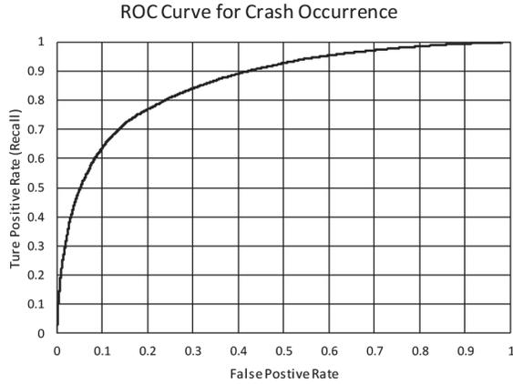
Figure 4: Receiver operating characteristic curve for classifying crash occurrences.
