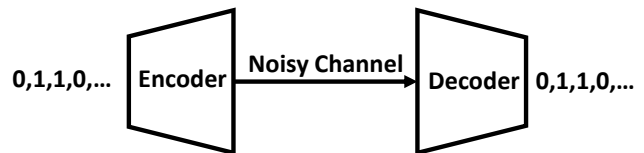
Figure 1: A channel codec uses one encoder and one decoder to recover the information after noisy transmission.
