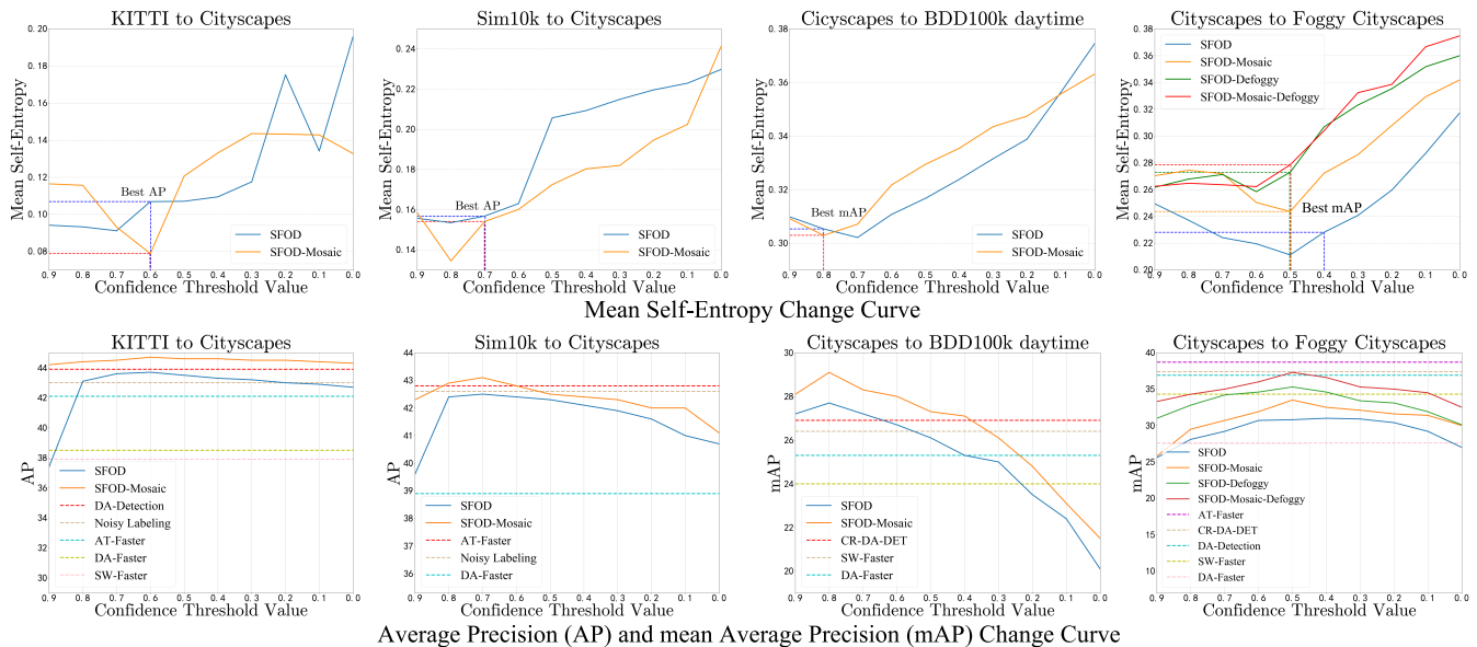
Figure 7: The curves of mean self-entropy and the corresponding AP or mAP vary with confidence threshold in four adaptation tasks. It can nearly search the best mAP via SED.
