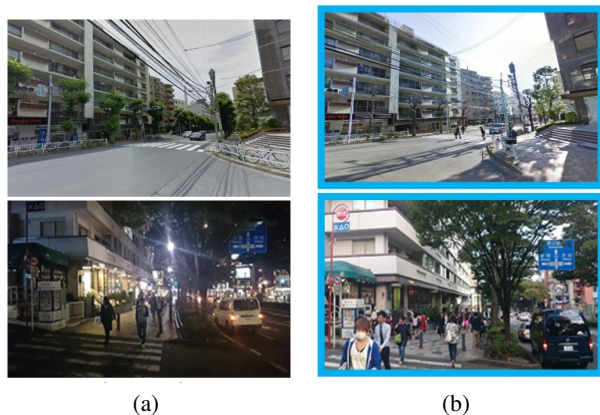
Figure 1. DenserNet can correctly perform visual localization under challenging conditions. Despite environmental variations (such as pedestrian or vehicle occlusions, illumination changes, and seasonal changes), DenserNet can find the location (a) from the database based on the query (b).
