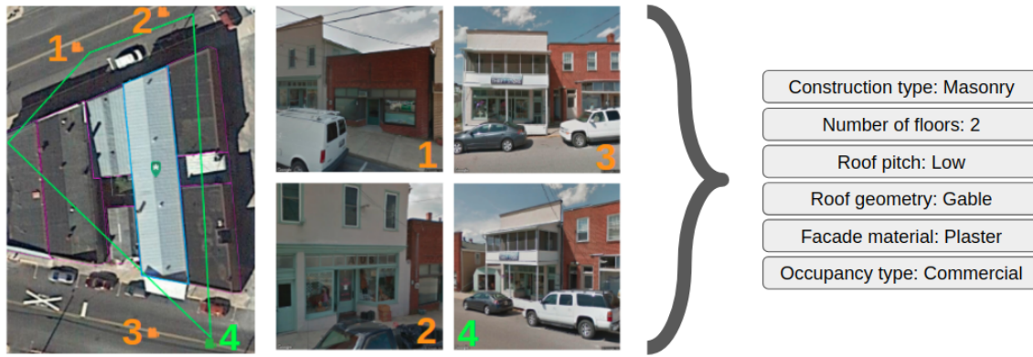
Figure 1: An example of a challenging building scene in our dataset. We aim to answer multiple questions about the building, and the answer to each lies in a different input image. The green mark represents the source location of the bottom right image number 4, while the green rays represent its field of view. The building of interest is marked with a green pointer on the top-view image, and it is the white one on the side view. The shading on the top-view image reveals that the roof is not flat, and the geometry is a gable. The front wall occludes most of the roof, but we can still infer its low pitch. The first image is not precisely calibrated and could suggest wrong answers, but combining information from all the sources should prevent it.
