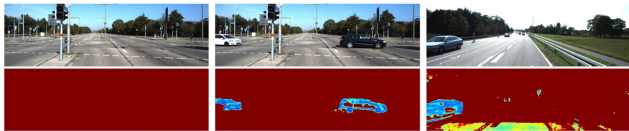
Figure 5: Visualization for our occlusion maps. The ego-motion is stationary in the first two columns while dynamic in the last column. For stationary scenarios, only moving objects are detected. In dynamic scenarios, occlusions (e.g., caused by traffic signs), moving objects, and truncation are detected at the same time. Our occlusion map \hat{\mathbf{K}}_s helps to remove ambiguous areas in view synthesis, thereby improving both the depth prediction and relative pose estimation.
