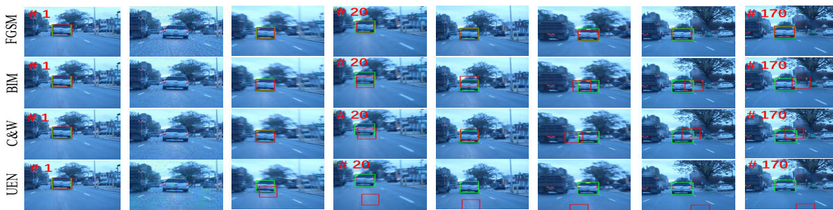
Figure 2: Comparative generated adversarial examples (the second column) and attacking results of UEN and other adapted baselines for non-target attacks against SiamRPN++. Green boxes mean the ground-truth, while red boxes denote the tracker’s output and numbers represent the frame index. UEN makes the tracker fail within 20 frames.
