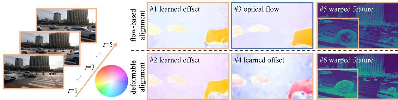
Figure 1: The learned offsets in both flow-based alignment (#1) and deformable alignment (#2, #4) have similar patterns as optical flow obtained using a deep learning-based optical flow estimator (Sun et al. 2018) (#3). The offset diversity allows deformable alignment to learn complementary offsets (#4), which effectively alleviate the occlusion problem and reduce warping errors. As a result, the warped feature after deformable alignment (#6) contains more details than that with flow-based alignment (#5) (see details of the car wheel).
