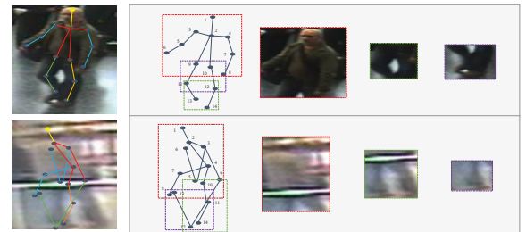
Figure 3: Samples of 14 landmarks detected on iLIDS-VID. Landmarks of the first line are detected successfully and image of the second line with low resolution and blur failed to detect.
