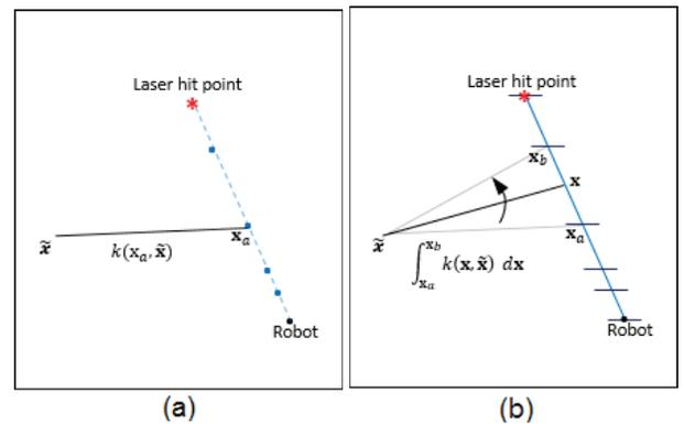
Figure 2: (a) points are used in typical continuous occupancy mapping (b) using a collection of line segments instead of points
