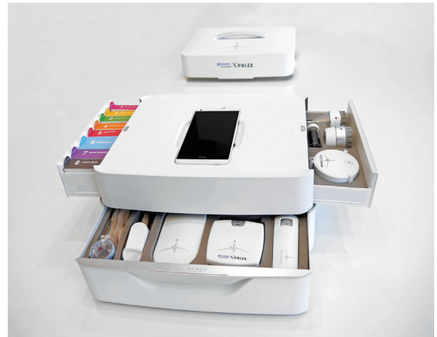
Figure 1: XPRIZE DeepQ Tricorder. DeepQ consists of four compartments. On the top is a mobile phone, which runs a symptom checker. The drawer on the right-hand-side contains optical sense. The drawer on the lower-front contains vital sense and breath sense. The drawer on the left-hand-side contains blood/urine sense. The symptom checker guides a patient on which tests to conduct.
