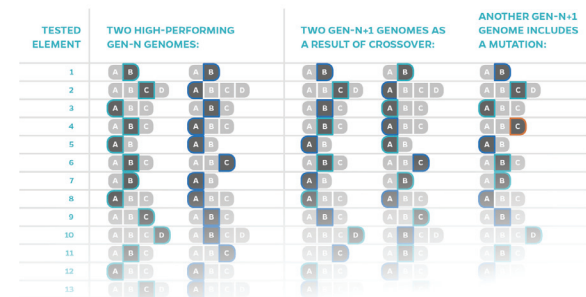
Figure 2: Genetic Encoding and Operations on Web Interface Candidates. The pages are represented as concatenations of their element values with one-hot encoding. Crossover and mutation operate on these vectors as usual, creating new combinations of values.
