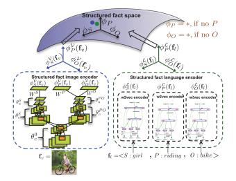
Figure 3: Structured Embedding Model (SEM). See Fig. 2 for the full picture.
