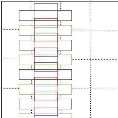
Figure 2: Illustration of default boxes for a 4\*4 grid. For better visualization, only a column of default boxes whose aspect ratios 1 and 5 are plotted. The rest of the aspect ratios are 2,3,7 and 10, which are placed similarly. The black (aspect ratio: 5) and blue (ar: 1) default boxes are centered in their cells. The green (ar: 5) and red (ar: 1) boxes have the same aspect ratios and a vertical offset(half of the height of the cell) to the grid center respectively.
