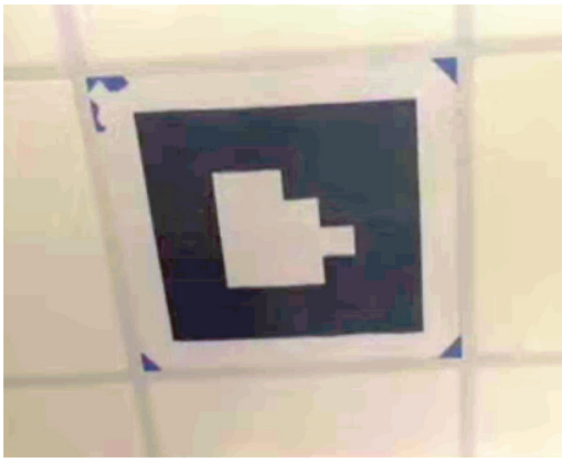
Figure 2: A ceiling mounted AR tag. These tags can provide accurate positioning information using the ar_pose ROS package. If the position of the tag is known within the room, one can obtain ground truth location data for a robot based on an image of the tag captured from a camera mounted on the robot.
