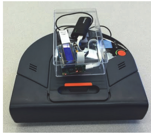
Figure 1: A Neato XV-21 with attached Raspberry Pi 2. Here, the camera is mounted forward-facing, however, for collection of ground truth data the camera should be mounted upward-facing.
