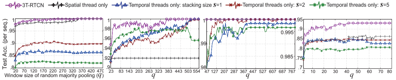
Figure 7: Mean accuracy as a function of window size for random majority pooling. Left to right: SD10, SPr10, BDH10, HCs10.
