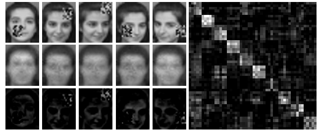
Figure 4: (a) Decomposition results of testing images on ORL database; the top five images are original images with 10% block corruption, while the middle five images are the low-rank recovery images and the bottom five images are corresponding to sparse noises including block corruption and facial expression changes; (b) Representations of testing images from the first ten classes on ORL database have classwise block-diagonal structure.
