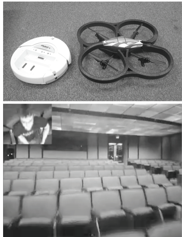
Figure 1. (top) the ARDrone beside an iRobot Create (bottom) a snapshot from the drone's outward and downward video feeds.
