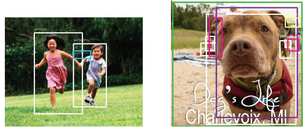
Figure 1: (left) YOLO model incorrectly predicts a car between 2 kids (in blue bounding box), and (right) a person is predicted in the large white bounding box. This paper automatically compiles such errors.
