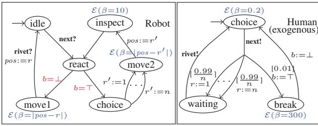
Figure 2: Illustration of automata-network encoding for the riveting application, with robot workflow of type (3b), and human workflow of type (1b) and (2a).  $\mathcal{E}(\beta=x)$  denotes the exponential distribution with mean  $x$ .
