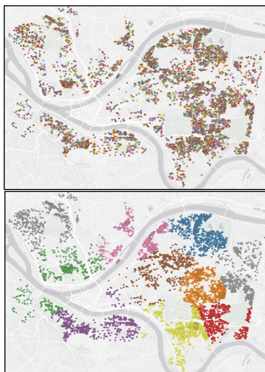
Figure 2: The difference between non-spatial (top) and spatial (down) cross validations. Points with the same color is to be considered as the validation fold for each iteration of the validation.
