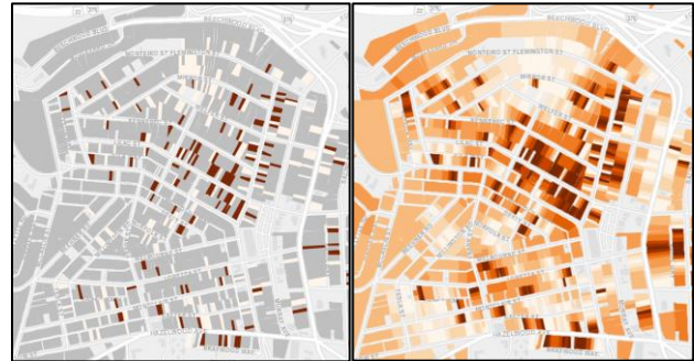
Figure 1: Example results of interpolating missing curb box inspections using the IDW technique with a power of 2. Training data are on the left and interpolations are on the right. Results are for the public portion of water laterals. Darker and lighter color indicates a higher or lower probability of lead, respectively.
