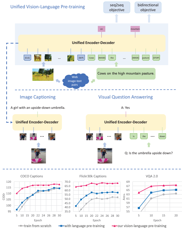
Figure 1: We propose a unified encoder-decoder model for general vision-language pre-training. The pre-trained model is then fine-tuned for image captioning and visual question answering. Thanks to our vision-language pre-training, both training speed and overall accuracy have been significantly improved on the downstream tasks compared to random initialization or language-only pre-training. All the results are evaluated on the validation set of the corresponding dataset.
