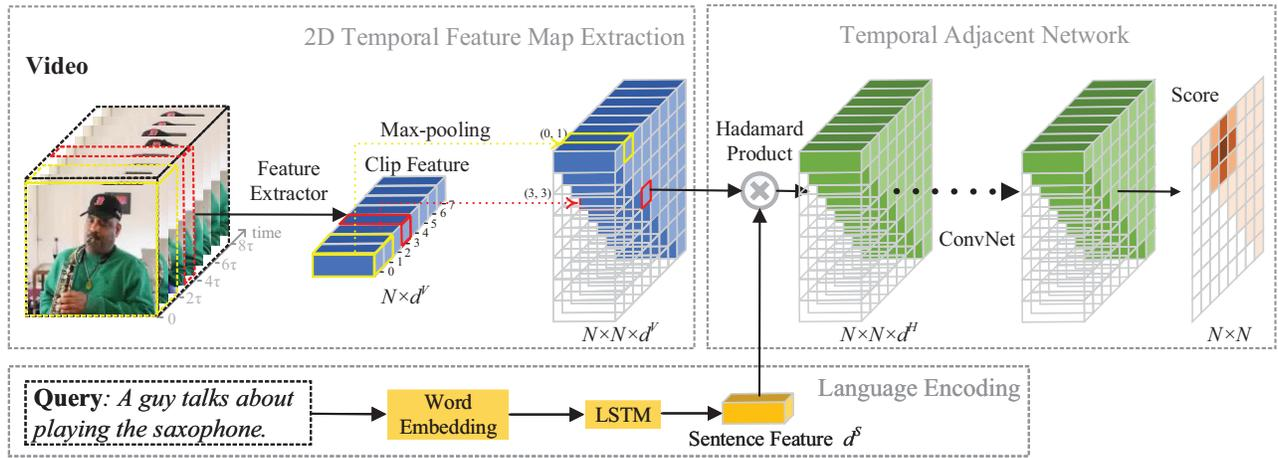
Figure 2: The framework of our proposed 2D Temporal Adjacent Network. It consists of a text encoder for language representation, a 2D temporal feature map extractor for video representation and a temporal adjacent network for moment localization.
