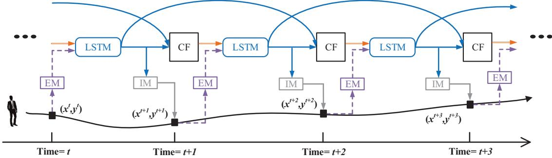
Figure 2: Overview of proposed CF-LSTM. 'EM' represents the extracting module, 'IM' represents the inference module, and 'CF' represents the cascaded feature module.
