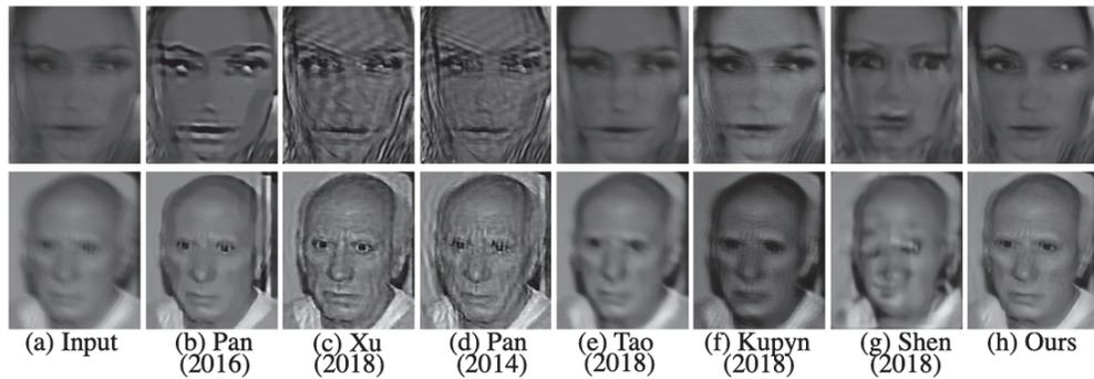
Figure 5: Visual comparisons with state-of-the-art on real blurry face images. The deblurred results of the proposed method have fewer artifacts and more details (best viewed on high-resolution displays).
