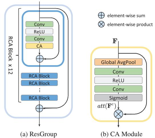
Figure 4: Illustration of ResGroup and CA module.
