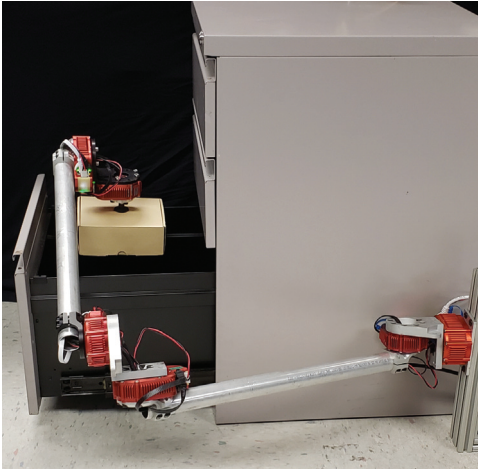
Figure 3: Top: An arrangement of modules (dark grey and red) with base located at the origin reaches a single workspace target position and tip axis (green point with arrow) without colliding with voxelized obstacles (grey cubes). Bottom: The physical modular robot matches the arrangement and environment.
