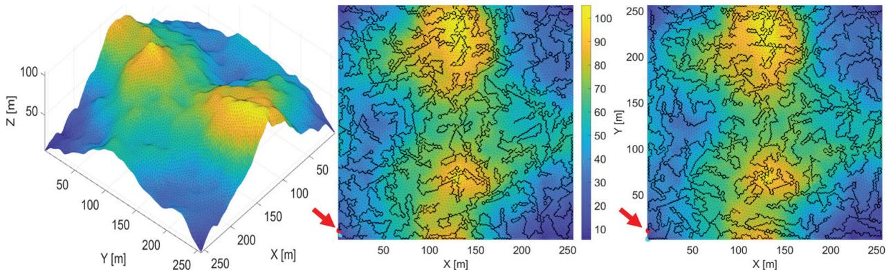
Figure 1: Left: A  $256m \times 256m$  random terrain considered in this study with  $80m$  elevation range; middle: the path generated using a grid; and right: the path generated without using a grid. The red arrow shows the starting point.
