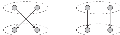
Figure 5: NOT gadget on the left, NOP gadget on the right.
