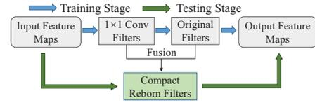
Figure 2: Using  $1 \times 1$  convolution to implement the reborn filters.
