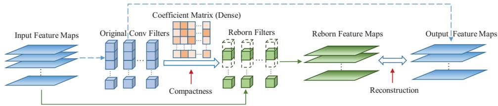
Figure 1: Pruning pipeline with reborn filters. Dashed blue line for original networks and solid green line for pruned networks. Reborn filters are developed by refining all the original convolutional filters in a layer, and making their input channels sparse (dashed green cubes) will induce pruning the input feature maps.
