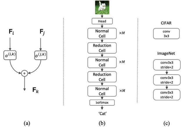
Figure 2: (a) The structure of the  $k$ -th block: taking two input feature tensors  $\{F_i, F_j\}$ , applying two separate operations  $\{o^{(i,k)}, o^{(j,k)}\}$ , and then combining them via element-wise addition as the output  $F_k$ . (b) Overview of building the network by stacking  $M \times 3$  normal cells and 2 reduction cells. (c) The head architectures used for CIFAR and ImageNet.
