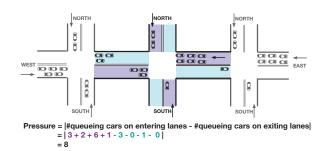
Figure 3: The illustration of intersection pressure.
