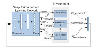
Figure 4: The framework of MPLight for multi-intersection signal control.
