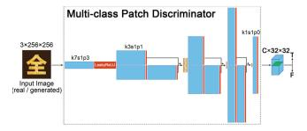
Figure 3: The architecture of discriminator D. The number of channels in output is the number of classes in the training set denoted as C. We calculate the loss by taking the channel corresponding to the class of the input.
