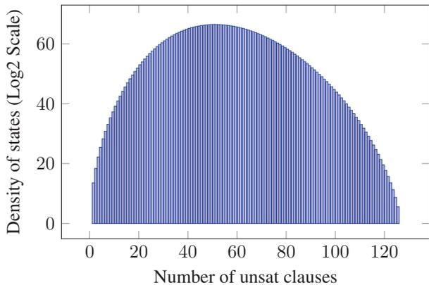
Figure 1: This example SAT problem has  $N = 100$  variables, and the clause density ratio  $\alpha$  is 4.0. The x-axis is the number of UNSAT clauses and the y-axis provides a numerical value for the number of assignments with the corresponding number of UNSAT clauses. The DOS over all possible variable assignments are captured in the histogram.
