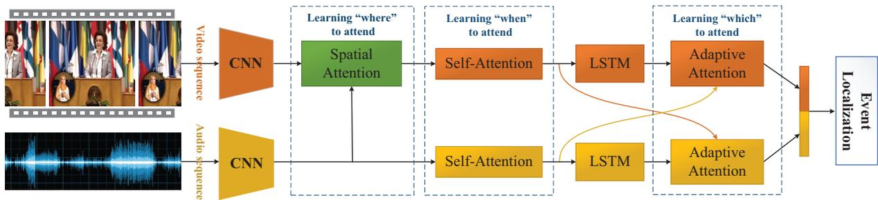
Figure 2: The diagram of the proposed cross-modal network for audio-visual event localization. The two modality-specific CNNs first process the corresponding audio and video into respective feature maps, then these feature maps are fed into three modules that automatically learn “where” (Spatial Attention Module), “when” (Global Context-aware self-Attention Module) and “which” (Cross-Modal Adaptive co-Attention Module) to attend for event localization.
