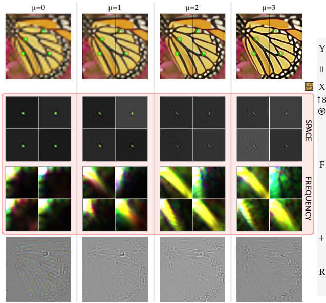
Figure 7: Output images for 8\times upscaling using different numbers of back-projections \mu . The network was trained with \mu = 2 fixed. The effective filters are shown together with their frequency response (FFT).
