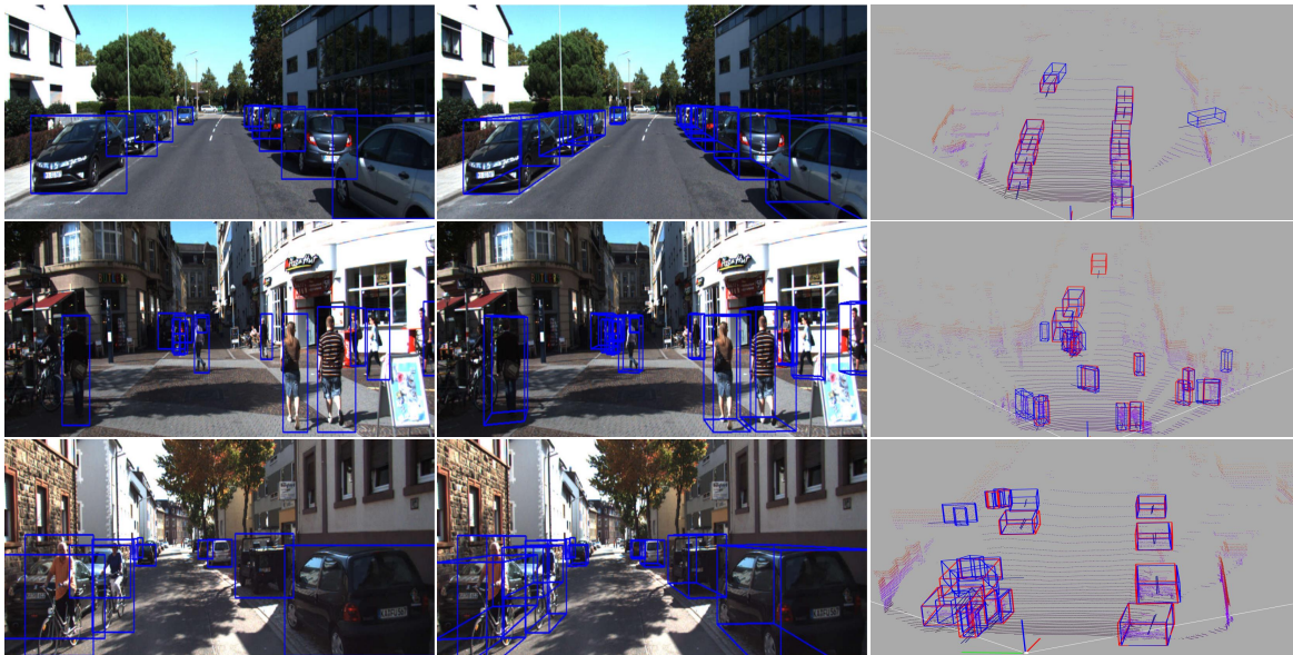
Figure 4: The visualization results for 3D object detection on KITTI validation set. The first column shows the 2D detection results on 2D images. The second column displays the 3D boxes that are projected on the 2D image. The last column demonstrates our 3D detection results on Lidar. The groundtruths are in red and the predicted boxes are in blue.
