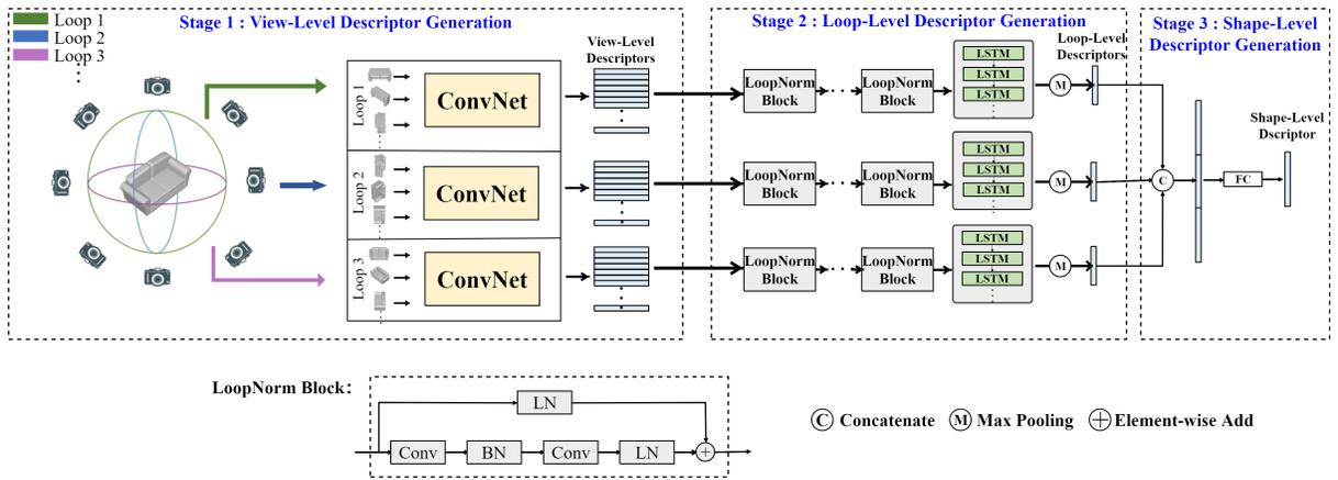
Figure 2: The Multi-Loop-View CNN framework for 3D shape retrieval. LN in LoopNorm Block denotes Loop Normalization and BN denotes Batch Normalization. The proposed MLVCNN contains 3 stages, during which it gradually obtains the descriptor from local descriptor of view-level, to more global descriptor of loop-level and shape-level.
