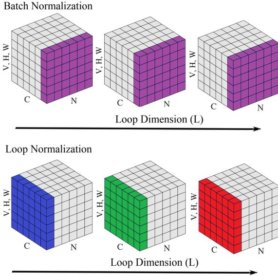
Figure 3: Batch Normalization(Top) and Loop Normalization(Bottom). In each row, cubes represent the input 6D tensor of (N,C,L,V,H,W) and each cube represents the sub-tensor sharing the same loop index in the input feature map tensor. In BN, pixels sharing the same channel(marked in purple) are normalized together. In LN, only pixels sharing the same channel and loop(marked in blue, green and red, respectively) are normalized together.
