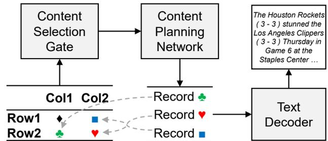
Figure 1: Block diagram of our approach.
