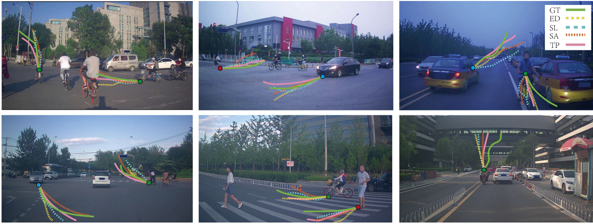
Figure 5: Illustration of our TrafficPredict (TP) method on camera-based images. There are six scenarios with different road conditions and traffic situations. We only show the trajectories of several instances in each scenario. The ground truth (GT) is drawn in green and the prediction results of other methods (ED,SL,SA) are shown with different dashed lines. The prediction trajectories of our TP algorithm (pink lines) are the closest to ground truth in most of the cases.
