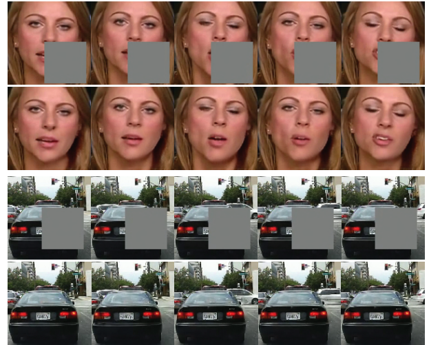
Figure 1: Video inpainting results by our approach. Row 1, 3: input frames with missing regions (shown in gray). Row 2, 4: our results. Note that the filled regions contain rich image details and are temporally coherent.
