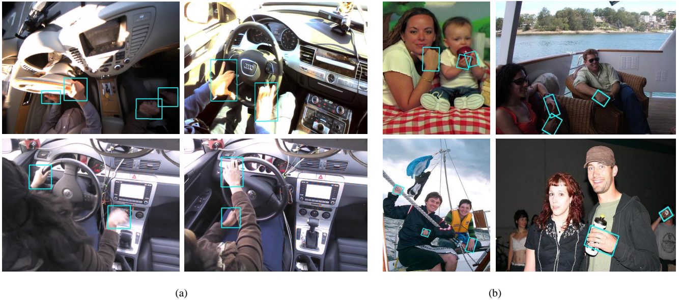
Figure 4: Detection examples of SIFCN with ResNet50 backbone. (a) Examples from the VIVA dataset. (b) Examples from the Oxford dataset.
