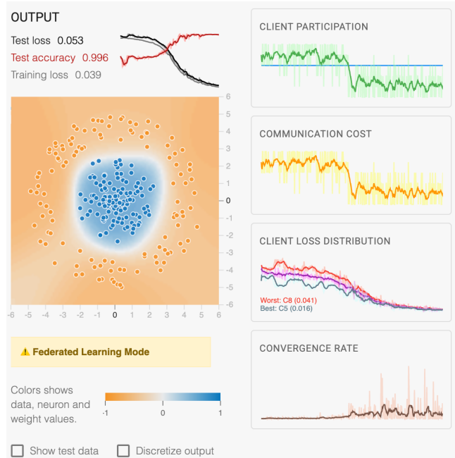
Figure 3: Simulated increase in client dropout halfway through training, with visualizations of Client participation , Comms cost (scales with no. of clients), Client loss distribution (max, mean, min), and Convergence rate .
