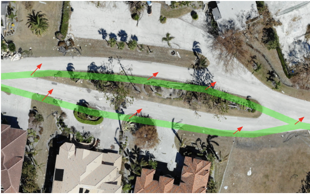
Figure 5: Example of a road line (colored in green) that is unaligned with the source imagery. Red alignment vectors show the transform necessary to align each vertex.
